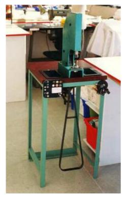
KPR1 is a foot operated ratchet press. It is supplied complete on a stand which incorporates two side trays for stud part storage.
